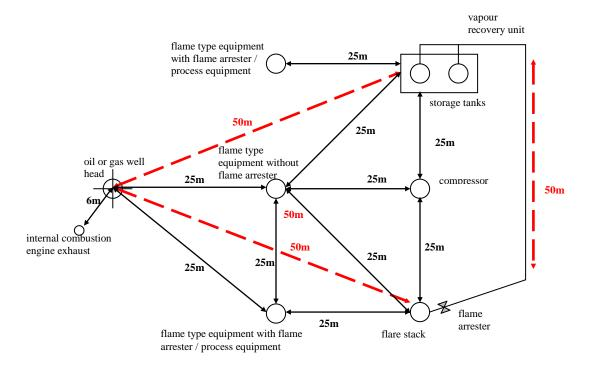
Dashed (Red) Line = 50 metres, Solid (Black) Line = equal to or greater than 25 metres, No smoking within 25 metres of well head, separator, oil storage tank or unprotected source of ignitable vapour
